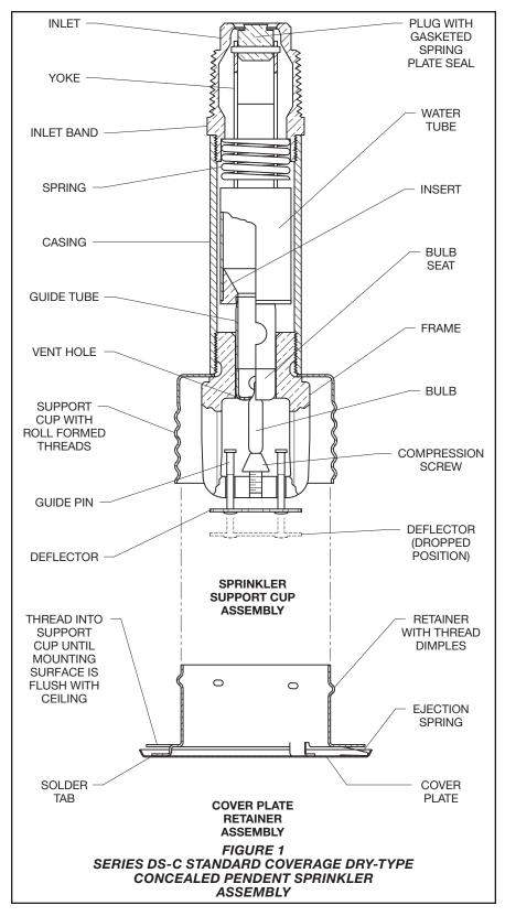
The compressed spring is then able to expand and push the water tube as well as the guide tube outward. This action simultaneously pulls inward on the
